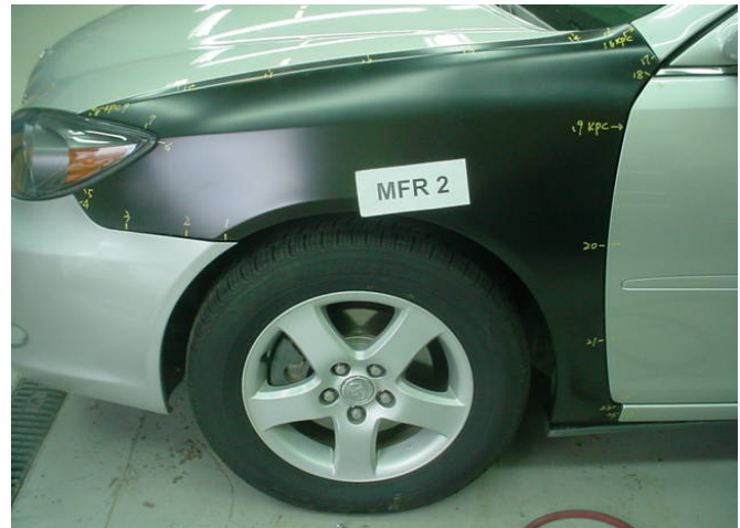
Diagram and corresponding photo of fender with checking fixture/VTF measurement points and mounting rail holes identified.
