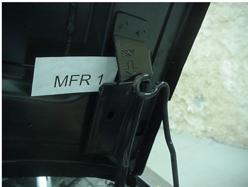
Faulty hinge prevents hood rod from safely engaging.
