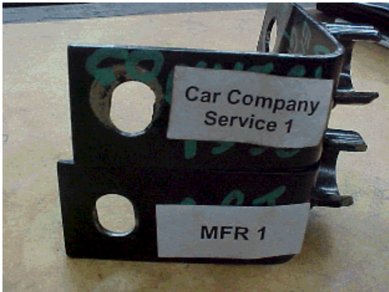
Faulty hinge bracket prevents tailgate from being installed.
