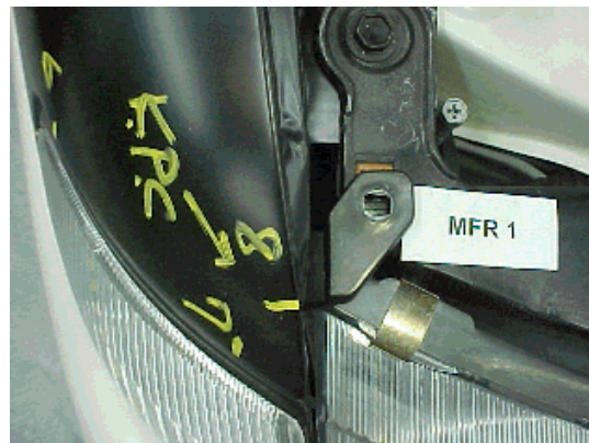
Non-certified AM fender incorrectly shaped/constructed. Corner lamp cannot be mounted.
